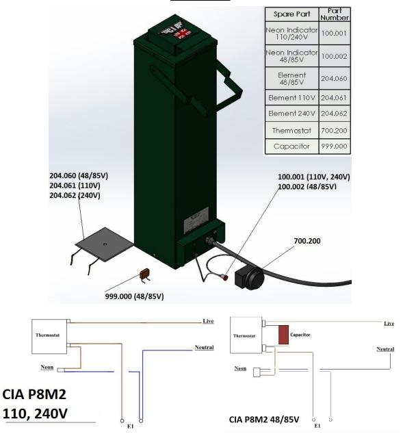
48/85V Versions are fitted with a capacitor between the thermostat terminals
