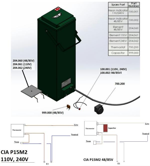
48/85V Versions are fitted with a capacitor between the thermostat terminals
