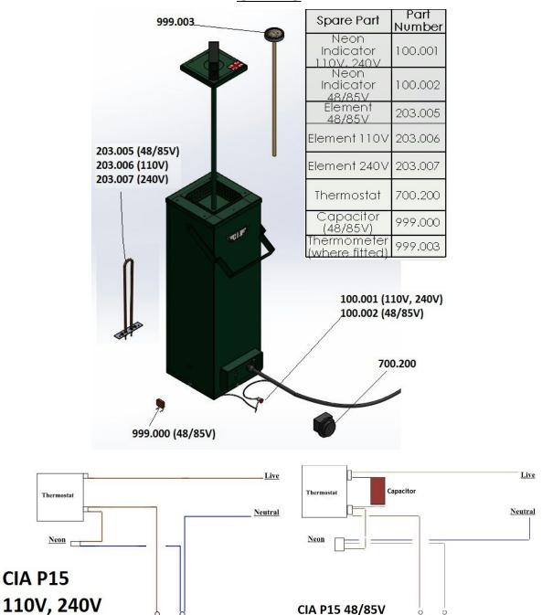
48/85V Versions are fitted with a capacitor between the thermostat terminals
