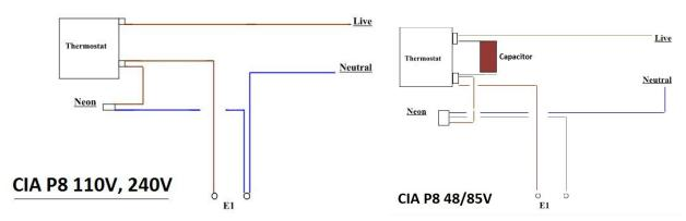
48/85V Versions are fitted with a capacitor between the thermostat terminals
